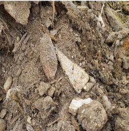
Suspected Asbestos Containing Materials (ACM) on tracking route between TP103 & TP104
