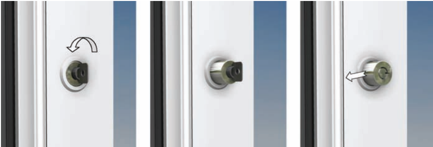
Figure 33 To unlock the centre plunger lock, turn the key until the plunger pulls back. To lock, once the sliding door is closed, simply push the plunger closed.
