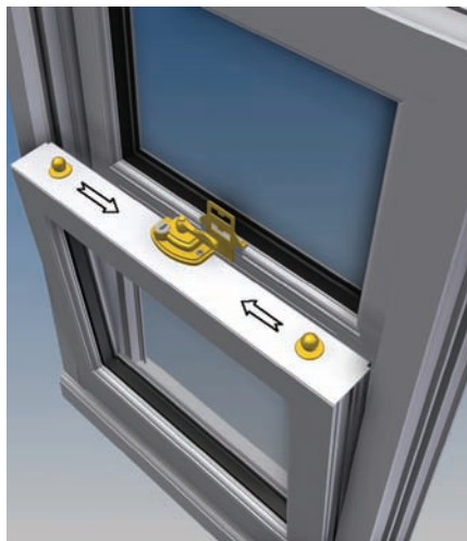
Figure 14 To clean the outside panes, slide the sash open about 100mm and pull back the jamb catches by sliding the tilt knobs inwards on the top of each sash. The weight of the windows will be supported on a support arm.
