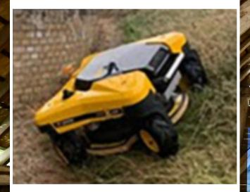
can cut vegetation to a height of up to 10 centimetres and at angle of 55 degrees, helping staff to cut difficult-to-reach spaces. The machine was paid for by the parks improvement fund and is proving to be more cost-effective than traditional methods.
